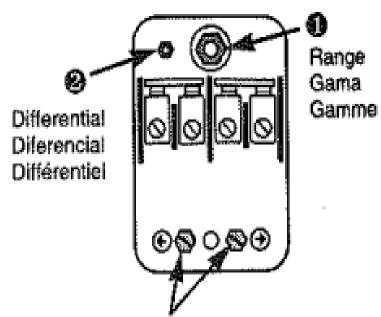
Grounding provisions: #10-32 screws. Torque screws to 15–20 lb-in (1.7–2.3 N•m).
